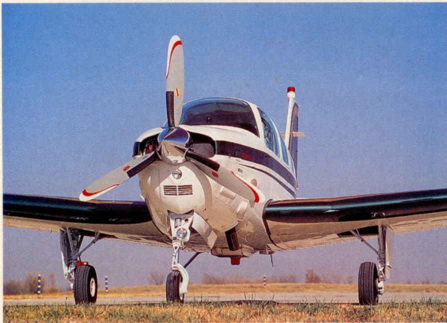
The B36TC is spotted by its lack of cowl flaps, single exhaust stack, and longer wings. The large scoop on the side of the cowl is the inlet for the heater. Raytheon recently switched to Hartzell propellers for all of its prop-driven airplanes from the Bonanza to 1900D airliner.
