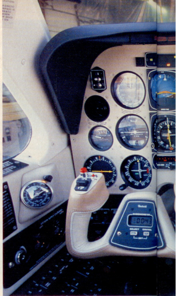
The extensive standard avionics package brings added capability yet reduced weight to the B36TC. Included are three-axis autopilot, ADF, DME, and dual IFR GPS mapcoms.
